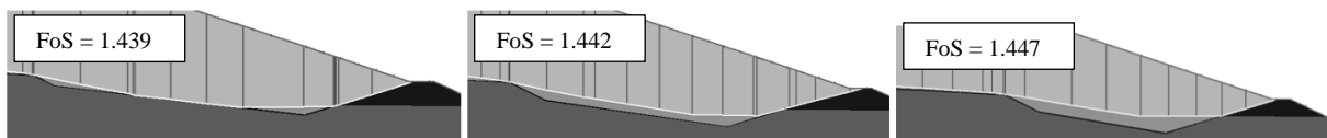
Figure 9. Critical slip surfaces for shear keys of 2 m (left), 4 m (middle), and 6 m (right) depths.
