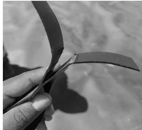
Figure 9. A cut out seam sample after a seam was failing NDT
