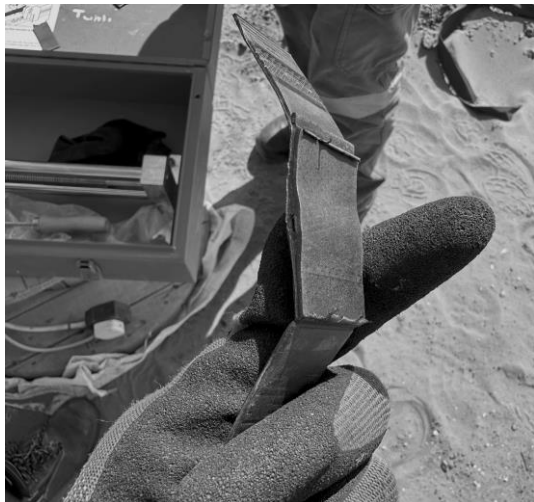
Figure 8. A destructive sample peel test (Pass)
