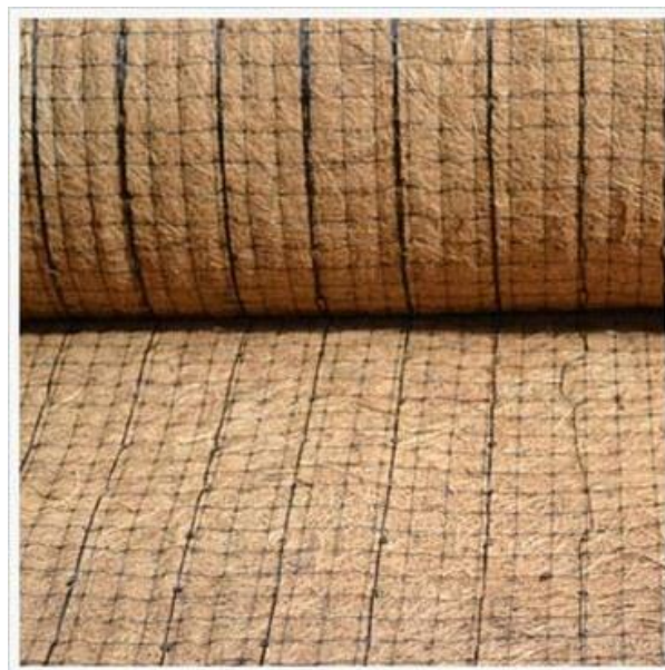
Image: Geoblankets manufactured out of jute (above) and coir (below)
