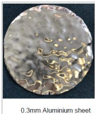
Figure 6. Damage to aluminum sheet under 250kPa or 500kPa applied Pressure.
