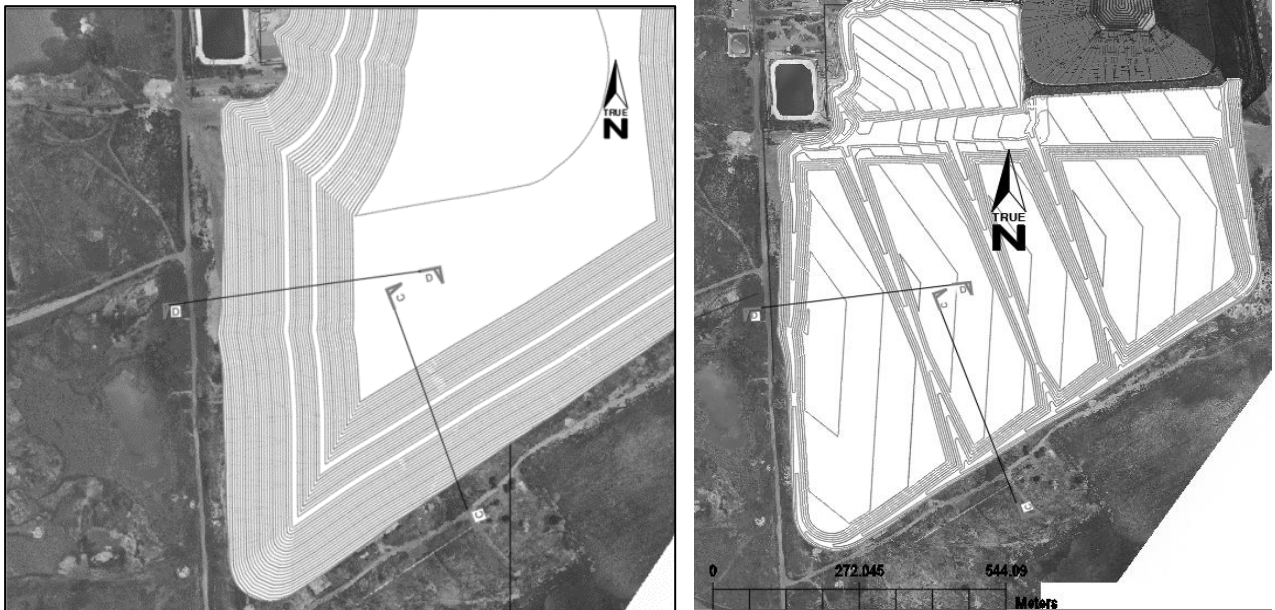
Figure 2: Plan view of the analyzed critical cross Section for Cell 13C and Cell 13D
