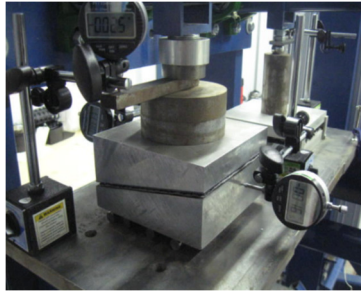
Figure 6: Representative photo of a conventional Creep with Shear Testing Apparatus.
