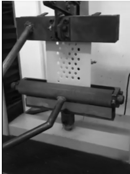
Fig 6. Tensile strength test
