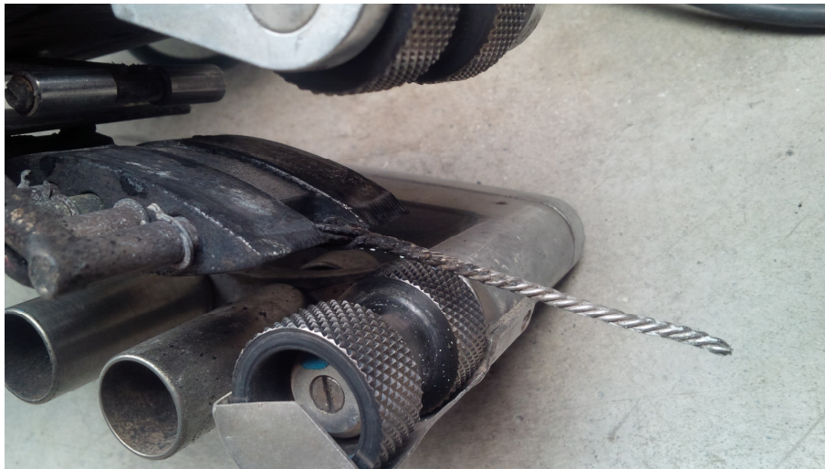
Figure 3: Groove bar fitted to wedge welder
