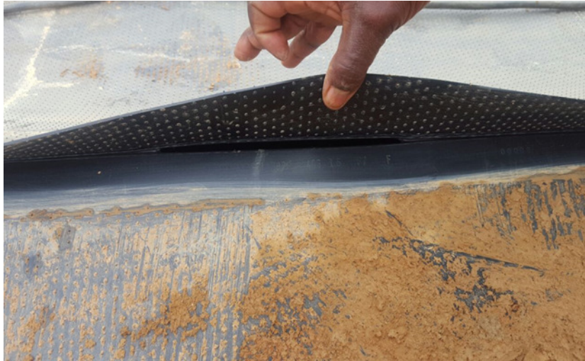
Figure 4: Slit created in base geomembrane of a wedge weld.
